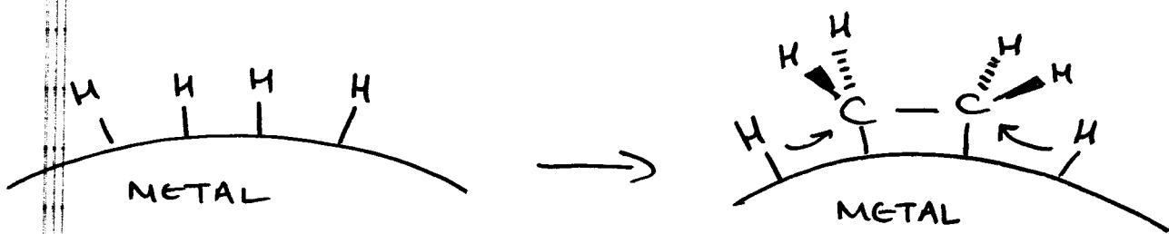
MINOR PRODUCTS RESULT FROM ISOMERIZATION OF THE ALKENE ON THE METAL CATALYST
