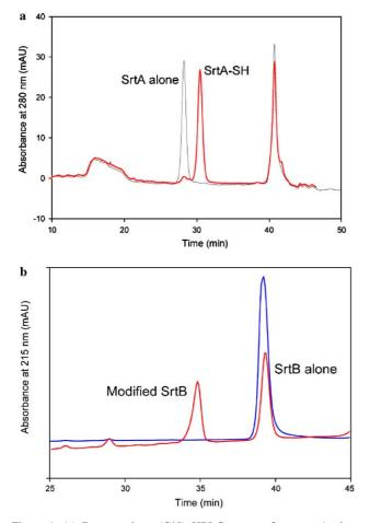
**Figure 1.** (a) Reverse-phase (C18) HPLC traces of sortase A alone (SrtA alone) and treated with a 10-fold excess of **11** (SrtA-SH). (b) Reverse-phase (C18) HPLC traces of sortase B alone (SrtB alone) and treated with a 5-fold excess of **17** after 12 h at pH 7 (modified SrtB).
