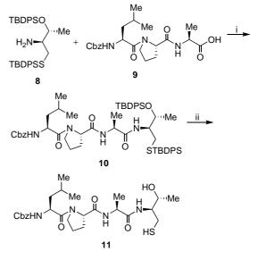
Scheme 2. Reagents and conditions: (i) EDCI, DMAP, HOBt, CH<sub>2</sub>Cl<sub>2</sub>,  $0 \, ^{\circ}C \rightarrow 23^{\circ}C$ , 2 h, 86%; (ii) TBAF, THF, 23  $^{\circ}C$ , 3 h; AcOH, 23  $^{\circ}C$ , 5 min, 70%.
