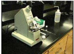
The refractometer is often stored with a piece of tissue in the prism assembly to keep the prism glass from being scratched. Open the prism assembly and remove the tissue.
