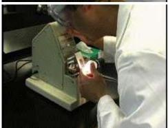
Close the prism assembly and turn on the lamp using the switch on the left side. (On some models the switch may be in the power cord.) Adjust the lamp so the light shines on the prism and look through the eyepiece.
