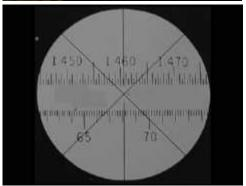
To read the index of refraction, depress the switch on the left hand side of the refractometer until you see the scale through the eyepiece. This is a view of what the scale will look like. The upper scale indicates the index of refraction. By carefully interpolating you should get 4 decimal place accuracy. You may want to pause the video and read the value now. The example shown here has a Refractive index of 1.4606.
