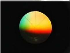
If you are close to the index of refraction of your sample you should see that the view in the eyepiece shows a dark region on the bottom and a lighter region on the top. If you do not see a light and a dark region, adjust the handwheel on the right side of the instrument until you do.
