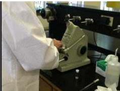
After you are finished, clean the refractometer. First use a tissue to dab away most of your sample. Then wash the prism with a little solvent, we usually use isopropyl alcohol. A dabbing motion rather than a rubbing motion is preferred to minimize the chances of scratching the prism.
