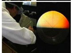
Once you have a crisp demarcation between the light and dark regions, use the handwheel on the right hand side to place this borderline exactly on the center of the crosshairs as shown. This is a view of what it should look like when correctly adjusted.
