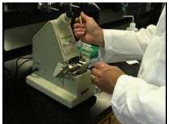
Use a pipet to apply your liquid sample to the prism, being careful not to let the glass pipet tip touch the prism since this may scratch the soft prism glass. Add enough sample to achieve a thin film across the whole prism, typically 3 to 4 drops.
