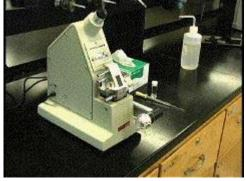
After you have finished cleaning the prism, place a clean tissue in the assembly. Before you leave make sure that the light has been turned off.
