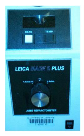
Locate the power switch on the right lower side in the front of the instrument. Turn the dial to  $n_D$  (middle). Place the lamp in the back on top of the prism. Now locate the eyepiece at the top of the instrument. You should see crosshairs with a shadow covering the lower part of the viewing range.
