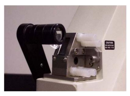
Close the hinged prism and return the light source to its original position (all the way down!).
