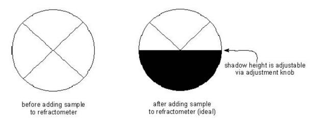
Using the adjustment knob (wheel) located on the right side of the refractometer, move the shadow until it intersects the crosshairs as shown above. Push the "READ" button and record the refractive index with four decimal places i.e. 1.3945. Then push the "TEMPERATURE" button to get the temperature reading (on the built-in thermometer). Adjust the refractive index to the standard 20 °C using the formula given above.
