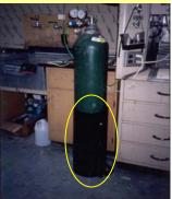
**Note:** For all *small gas cylinders* and specifically for those which require to be placed within the fume hood, use a frame casing (similar to clam shell) as shown in the pictures below:
