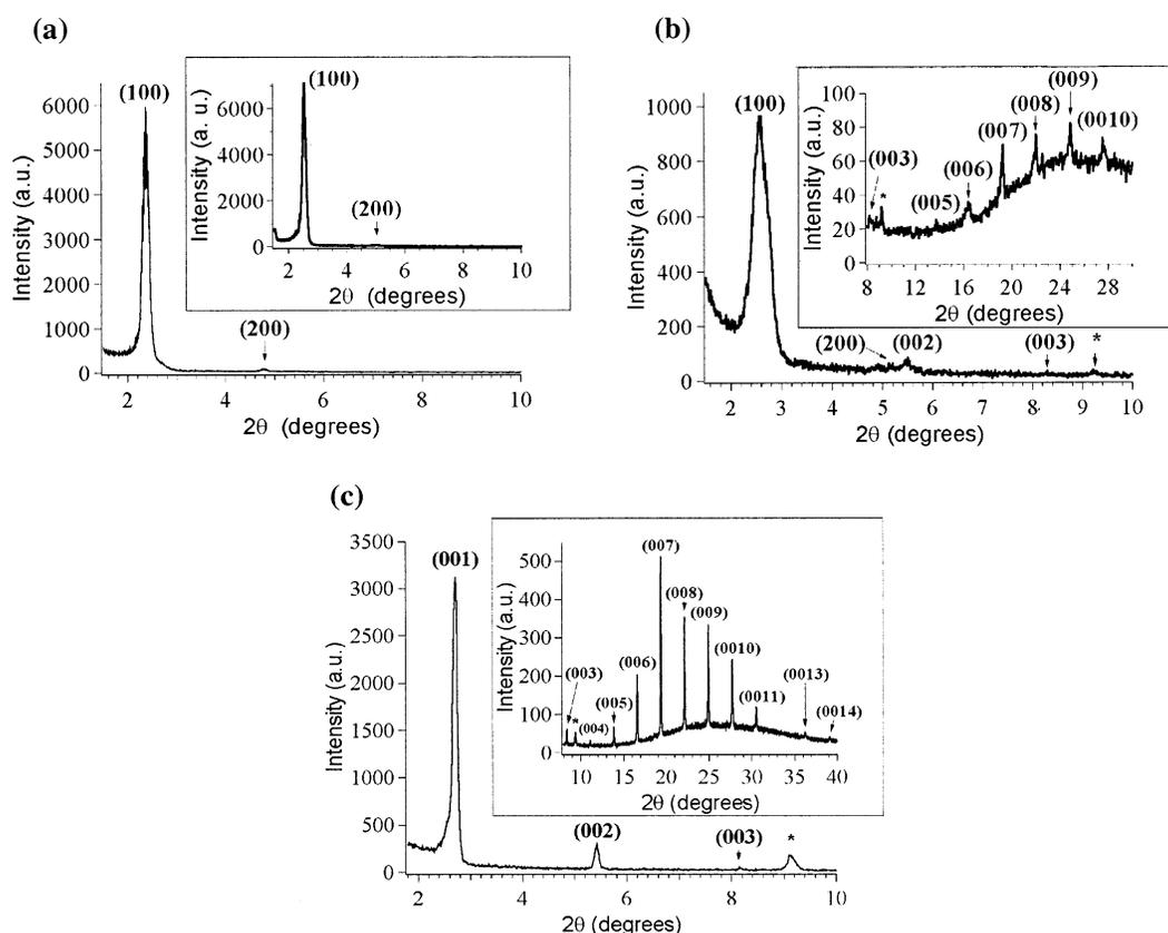
**Figure 4.** XRD patterns of the thin films with carbazole and a 3.5 wt % CTAB sol–gel silica film. (a) Thin film deposited on a glass substrate with 1:0.1 CTAB/carbazole. The inset corresponds to 1:0.41 CTAB/carbazole. Both have a hexagonal mesophase. (b) Thin film with 1:0.43 CTAB/carbazole; it has a mixed phase. (c) Lamellar phase for 1:1.2 CTAB/carbazole.
