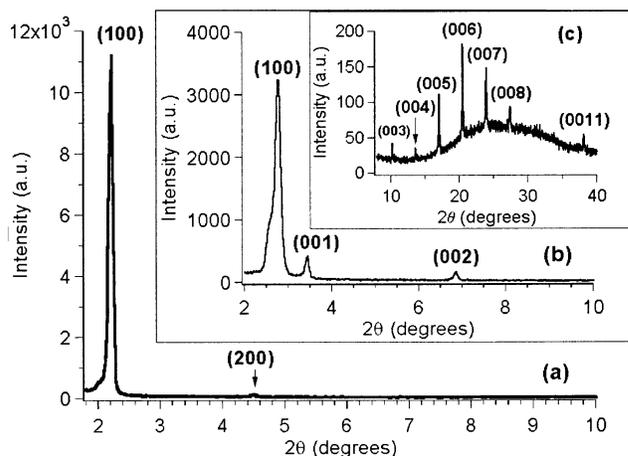
**Figure 2.** (a) XRD pattern of a 3.5 wt % CTAB sol–gel silica film that shows a hexagonal phase. (b) XRD patterns at a low angle of the mesostructured silica thin films with a CTAB/THF molar ratio of 1:84. (c) XRD patterns at a high angle from the same film as that in part b.
