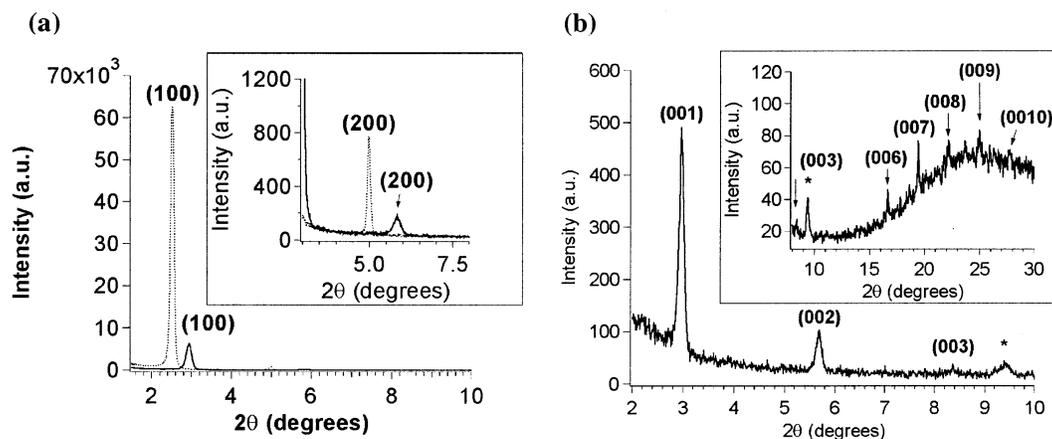
**Figure 3.** (a) XRD pattern of a 3.5 wt % CTAB sol–gel silica thin film with 1:20 CTAB/benzene (Table 2) before calcination (dashed line) and after calcination (solid line). The inset shows the (200) peaks. (b) XRD pattern of a 3.5 wt % CTAB sol–gel silica thin film with 1:0.62 CTAB/carbazole (Table 3) using benzene as the solvent. It shows a lamellar phase.
