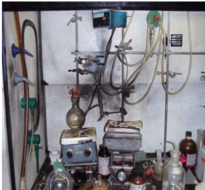
View 2 Fume hood after explosion
