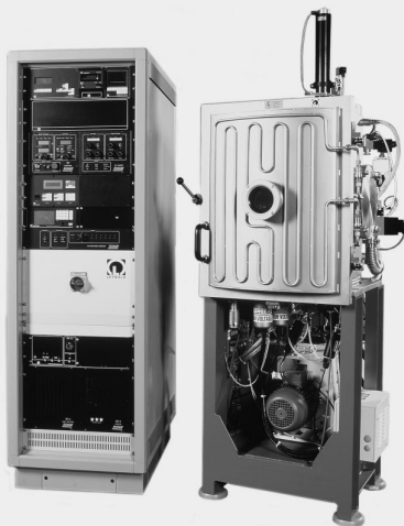
UNIVEX 450 B having a chamber diameter of 490 mm and with electron-beam evaporator with heatable and coolable chamber walls; with COOLVAC 3010 cryopump
