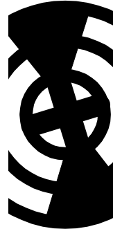
Rotation: poor polarizer alignment around Pockels cell
