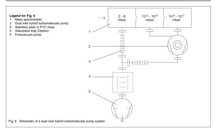
Ensure that the pump is sufficiently isolated against resonances (vibrations) generated by the forevacuum pump.
