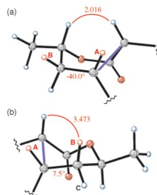
**Figure 3.** Tether-containing rings of the endo boatlike (a) and endo chairlike (b) transition states. Selected H–H distances (Å) and H–C–C–H dihedral angles are labeled.
