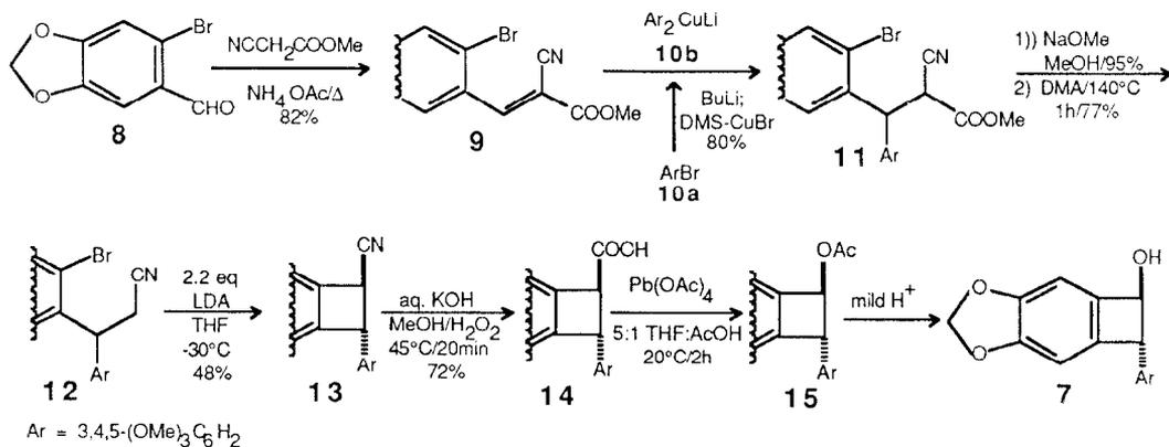
in good yield. This compound could be hydrolyzed under mild acidic conditions<sup>5</sup> to give the desired benzocyclobutenol **7**, thus completing an 8-step synthesis from **8** in fair overall yield.
