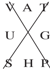
Figure 2.6. Each quantity at the center of a row or column is adjacent to its natural variables. The partial derivative with respect to one of the variables, with the other held fixed, is arrived at by following the diagonal line originating from that variable. Attach a minus sign if you go against the arrow.
