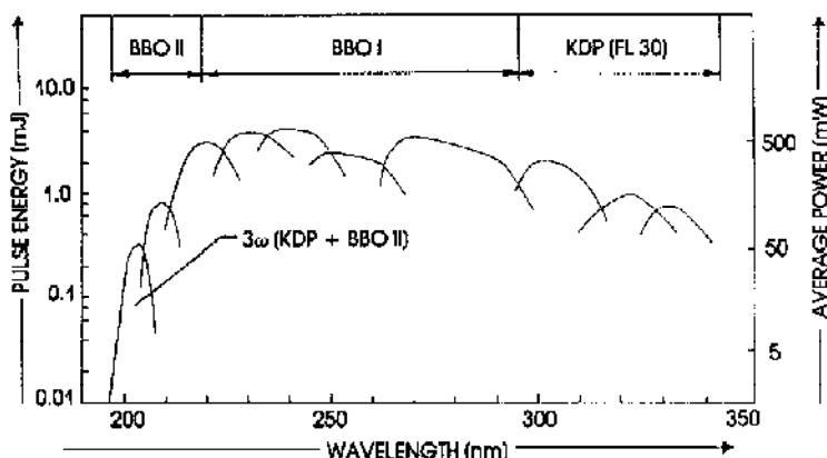
Excimer laser wavelengths range from 193 nm (ArF) to 351 nm (XeF). The strongest lines are at 248 nm (KrF) and 308 nm (XeCl). Most dyes have an absorption band at 308 nm. The result is that nearly the entire range of commercially available dyes can be pumped with a XeCl laser (see Figure 1).
